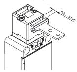
The head of this switch is equipped with an actuator with a wide range of travel. In this way the guard can oscillate along the direction of insertion (4.5mm) without causing unwanted machine shutdowns. This extensive travel is available in all actuators, in order to ensure maximum device reliability.
