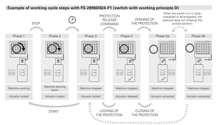
The GUARD CLOSING with de-energised solenoid brings the switch back in B state and then in A state in quick sequence.
