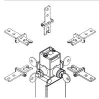
The head can be quickly turned on each of the four sides of the switch by unfastening the two fixing screws.
