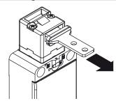
The strong interlocking system guarantees a maximum actuator holding force of  $F_{1max} = 1100 \text{ N}$  (head 96).
